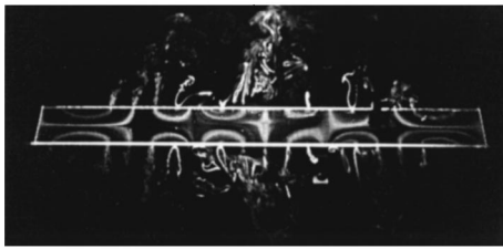
FIG. 3. Visualization of stream patterns using smoke sources and a sheet of laser light in a fluid layer under a beam vibrating with different mode shapes. Formation of jets are also apparent at the free edges. Air layer thickness is h_0 , A is the amplitude of vibration at an antinode, and f is the frequency of vibration.
